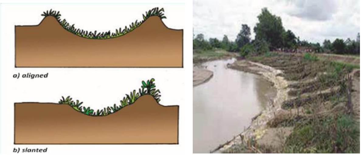
Figure 2.1.57: Variations of waterway cross-section and field application, showing (a) aligned waterway profile, (b) slanted waterway profile, and (c) stabilized field example.
