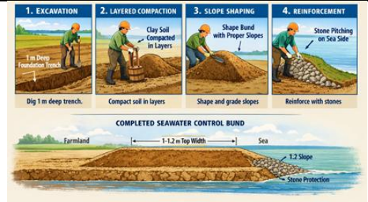
Figure 2.1.31. Step-by-step construction of a seawater control bund showing excavation, layered compaction, slope shaping, and reinforcement.
