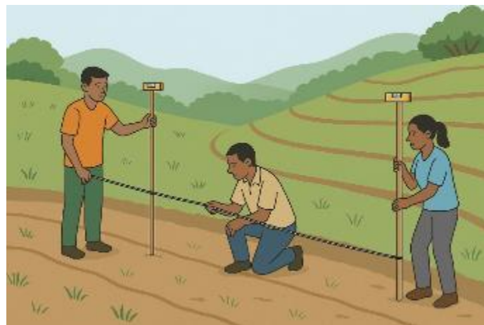
Figure 1.2.3. Field demonstration of contour marking using a line level, showing a three-person team operating along a gentle slope to identify points of equal elevation.
