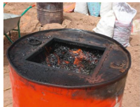
Figure 2.7.4 (inside view of drum kiln showing carbonization).
