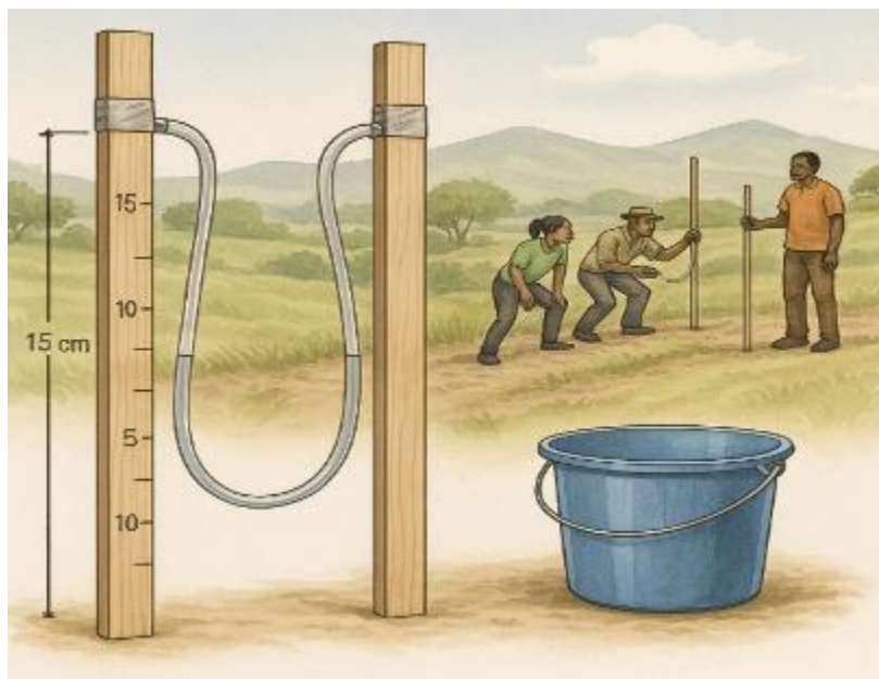
Figure 1.2.6. Illustration of a pipe level set-up showing two wooden scales connected by a transparent water-filled tube, demonstrating how equal water levels at both ends indicate points of equal elevation.
