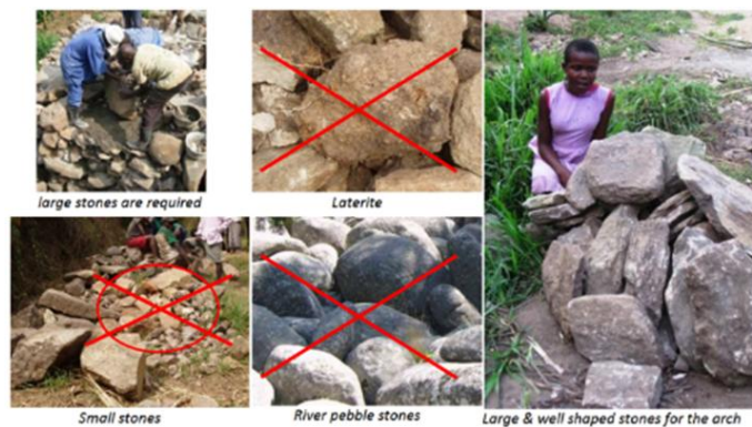
Figure 2.4.28. Suitable and unsuitable stones for arch construction
