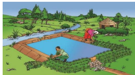
Figure 2.5.8. Vegetation establishment around a completed pond.
